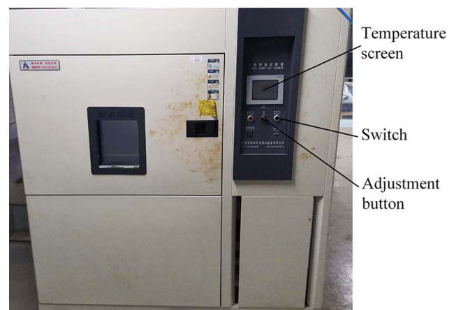
Fig. 9. (Color online) High and low temperature test box.
