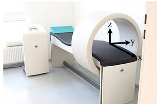
Fig. 1. (Color online) The device for physical therapy PMT quattro PRO with a marked coordinate system origin in the coil centre.
