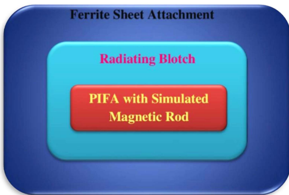
Fig. 1. (Color online) Amended Planar Inverted F- Antenna (PIFA) With Ferrite Sheet for SAR Reduction.
