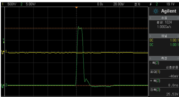
Fig. 5. (Color online) Output pulse waveform produced by a pulse generator.
