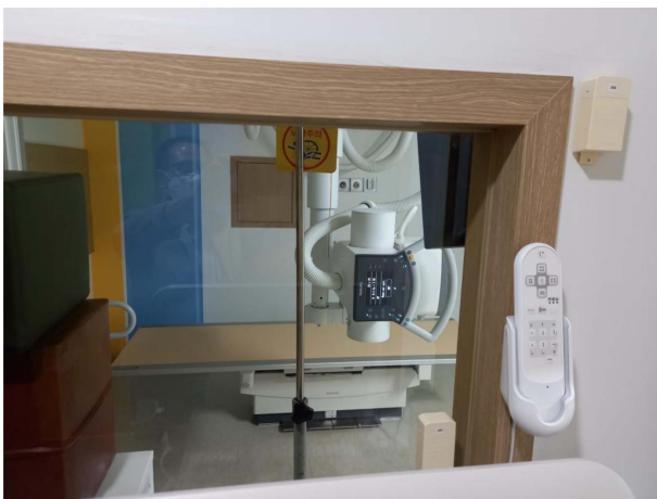
Fig. 3. (Color online) Glass dosimeter installation location for lead glass leakage dose measurement.
