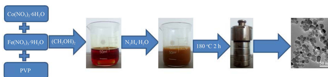
Fig. 1. (Color online) Schematic of the solvothermal process that was utilized in the preparation of \text{CoFe}_2\text{O}_4 nanoparticles.
