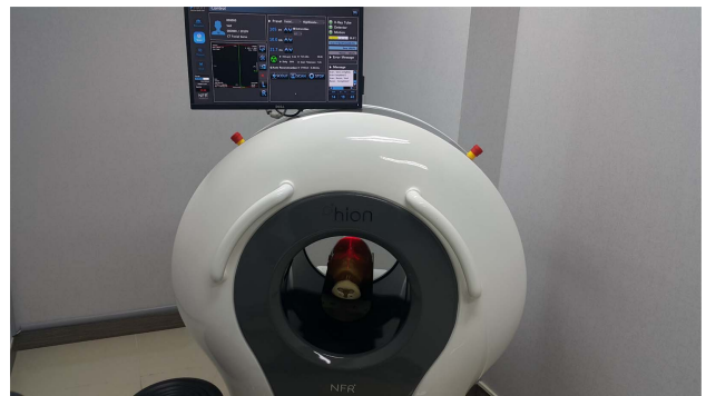
Fig. 2. (Color online) Mobile CT device and examination room for acquiring 2D, 3D medical images and measuring radiation doses.
