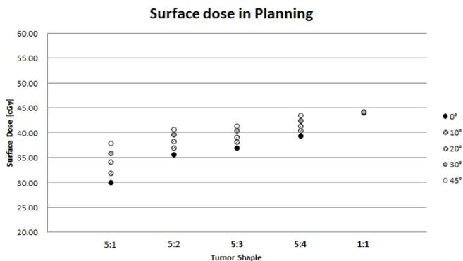
**Fig. 4.** Graphical representation of the surface dose value on the radiation treatment planning program according to the change in the shape of the tumor and the angle of the collimator.
