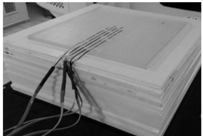
**Fig. 3.** Measure the surface dose according to the shape of the tumor and the change of the collimator angle after being located on the surface of the phantom using a MOSFET.
