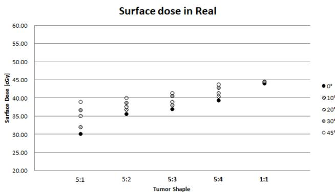
**Fig. 5.** Graphical representation of surface dose values using MOSFETs according to tumor type and collimator angle change.
