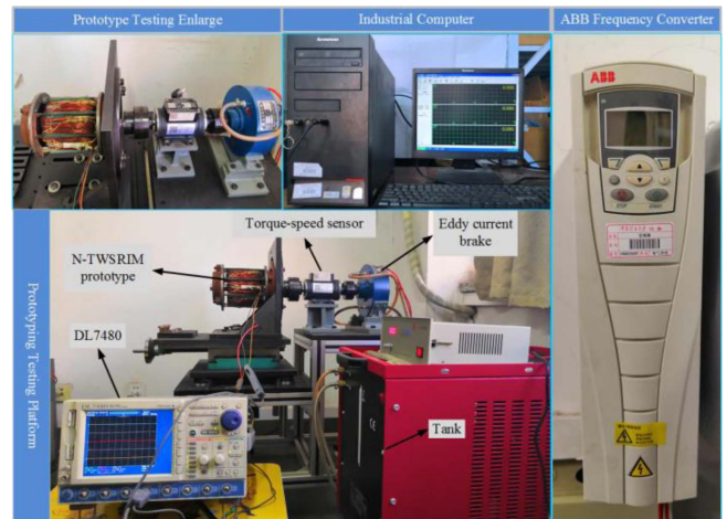
Fig. 12. (Color online) Prototype testing platform.
