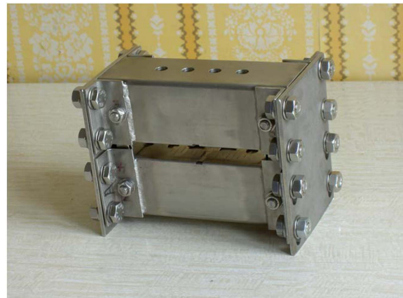
Fig. 4. (Color online) A compact device for the creation of a strong magnetic field in an air gap.
