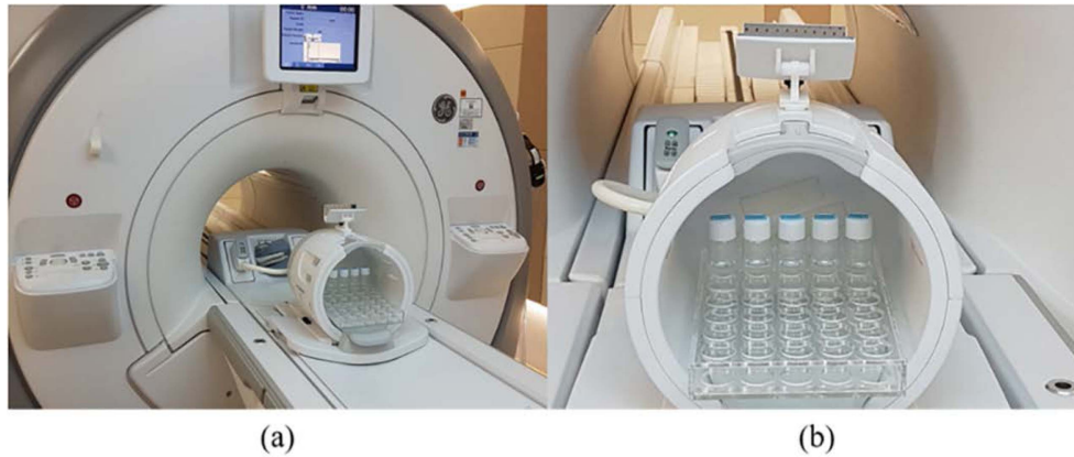
Fig. 5. (Color online) MR equipment (a) 3.0T GE discovery; (b) 32channel head coil.
