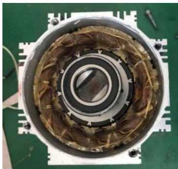
Fig. 7. (Color online) Prototype of the amorphous motor.
