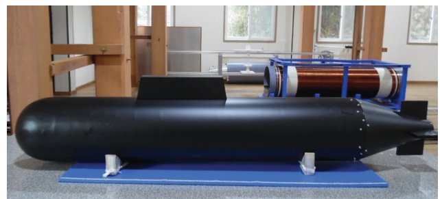
Fig. 7. (Color online) A photograph of a scaled model ship fabricated for verifying the purposed Flash-KD method.
