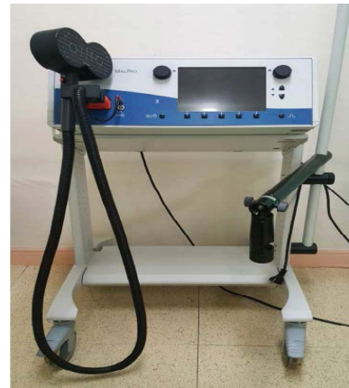
Fig. 2. (Color online) Appearance of the rTMS equipment used in this study (MagPro R30, Medtronic Inc., Skovlunde, Denmark).
