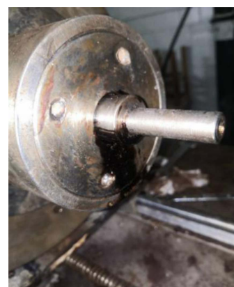
Fig. 14. (Color online) Common magnetic fluid seal failure.
