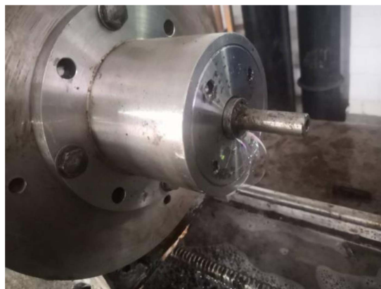
Fig. 13. (Color online) Diverging stepped magnetic fluid seal failure.
