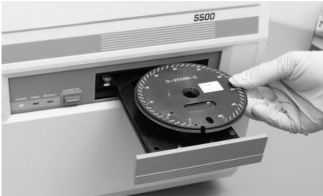
Fig. 2. The measured TLD device is an image of the process of extracting and comparing the glow curve expressed in the process of evaluating the dose through the TLD reader during the evaluation process.
