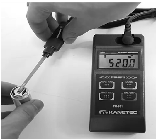
Fig. 3. Images measured for each condition using a magnetic field measuring tool to evaluate the exact magnetic field strength of the permanent magnet located during the experiment.
