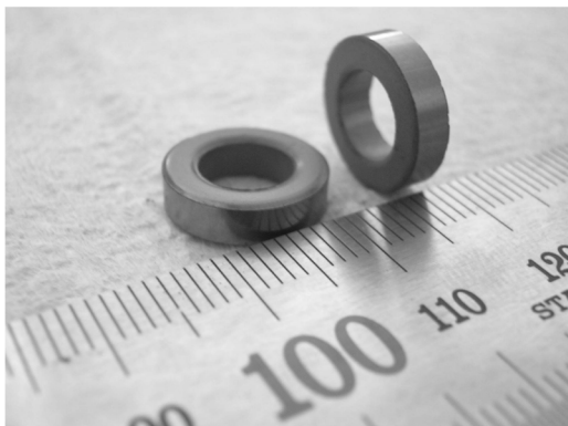
Fig. 3. The amorphous FeCrSiBC alloy powder cores using phosphate-coated powders prepared by cold-pressing.
