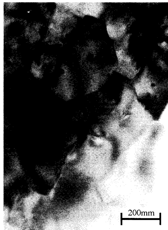
Fig. 5. TEM micrograph showing the microstructure of the optimally recombined material (solid HDDR-treated alloy B).
