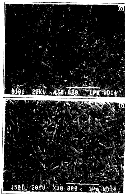
Fig.7 SEM micrographs of surface of barium ferrite thin films as a function of coating time.
