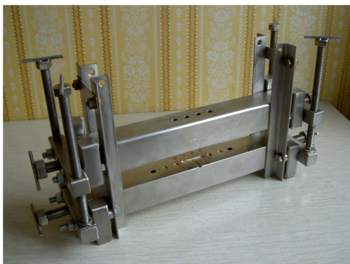
Fig. 4. (Color online) A device for placing NdFeB magnets into two opposing assemblies.
