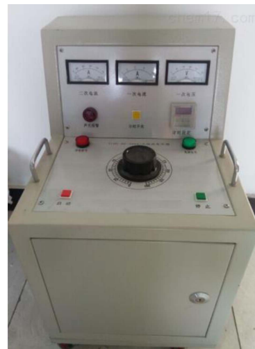
(b) High current generator (2000A)
