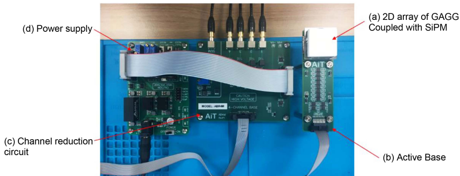
Fig. 2. (Color online) Photograph of (a) the 2D array of GAGG scintillator coupled with the SiPM, (b) active base, (c) channel reduction circuit, and (d) power supply.
