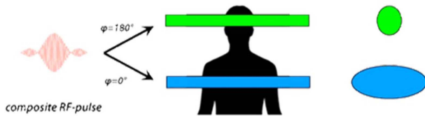
Fig. 1. (Color online) Multi-band Sensitivity (MB-SENSE) imaging. A complex RF-pulse simultaneously stimulates two slices, which are phase offset from one another by an amount that depends on the phase-encoding step (here 180^\circ ).
