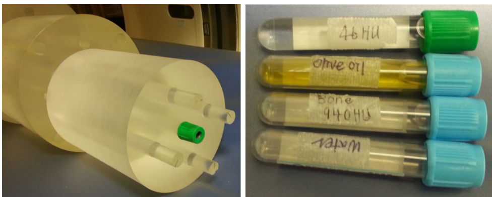
Fig. 2. (Color online) PMMA phantom used for measurements and plastic tube inserted containing water (0 HU), iodine (200 HU), \text{CaCl}_2 (1000 HU), and fat (-120 HU) contrast solutions.
