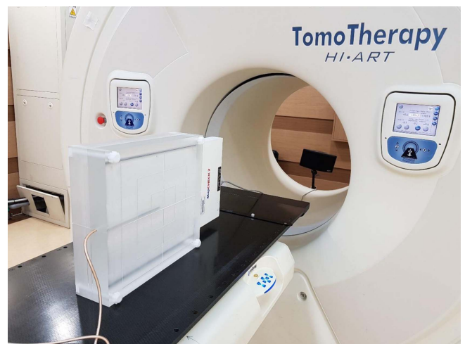
Fig. 5. (Color online) Experimental setup of multipurpose phantom in tomotherapy system.
