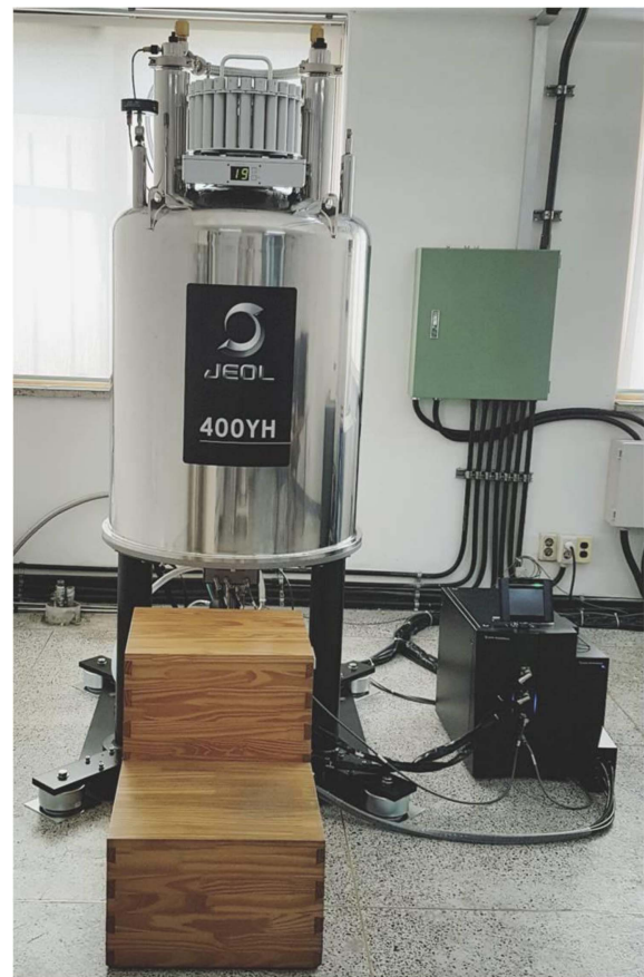
Fig. 1. (Color online) FT-NMR 400 MHz spectrometer used for measuring the total fluorine content.
