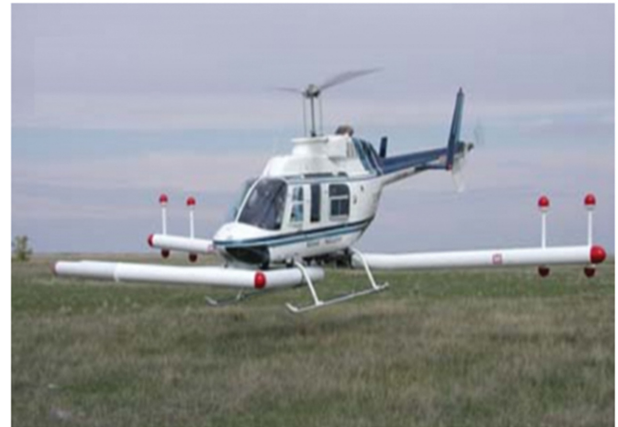
Fig. 7. (Color online) Helicopter carrying gradiometer type atomic magnetometers for UXO detection.
