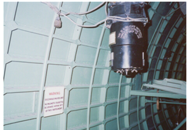
Fig. 3. (Color online) MAD method using using flux-gate magnetometer.
