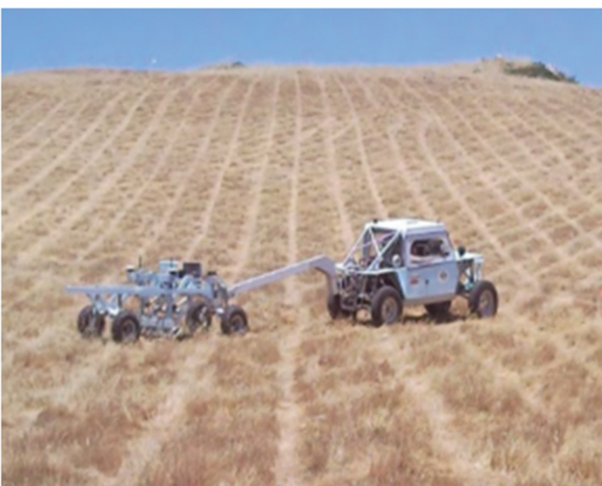
Fig. 6. (Color online) Trailer carrying atomic magnetometer for UXO detection.
