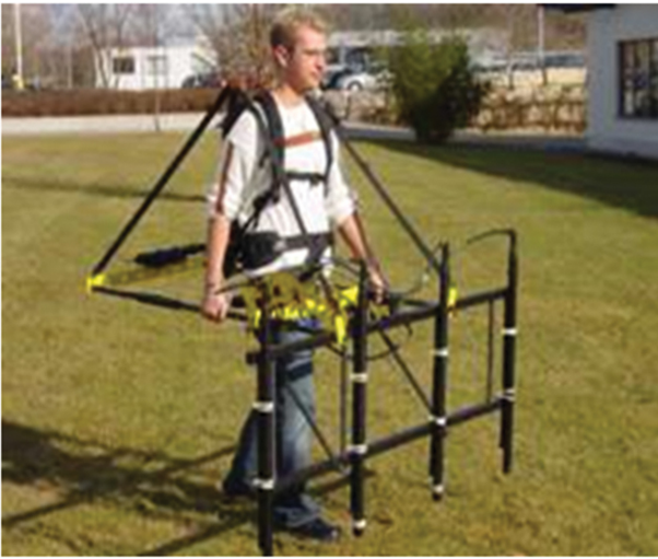
Fig. 5. (Color online) Hand carrying magnetic gradiometer with 1-axis flux-gate magnetometer for UXO detection.
