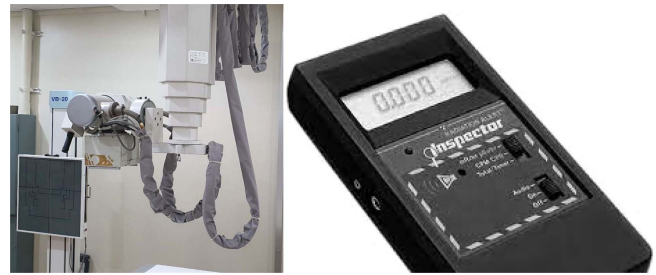
Fig. 1. (Color online) (Left) Image of DK2325R, a diagnostic electromagnetic radiation generator, and (Right) image of INSPECTOR, an electromagnetic radiation measurement device.
