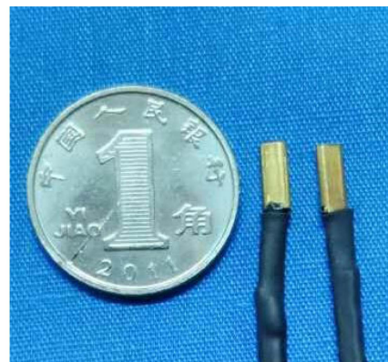
(b) Structure of the Hall probes
