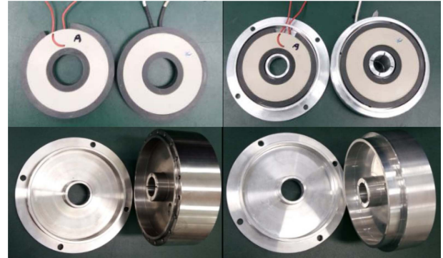
Fig. 8. (Color online) Fabricated coil, ferrite core, SUS304 housing, and Al6061 housing.
