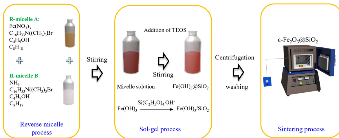
Fig. 1. (Color online) Schematic illustration of the synthesis of the \epsilon -Fe 2 O 3 phase.
