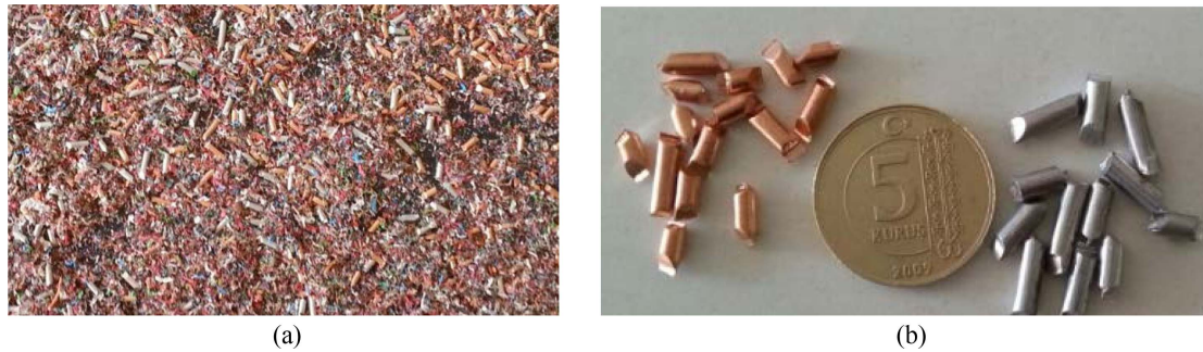
Fig. 6. (Color online) Granule cable waste (a) mixture cable waste with pvc (b) granule cable.
