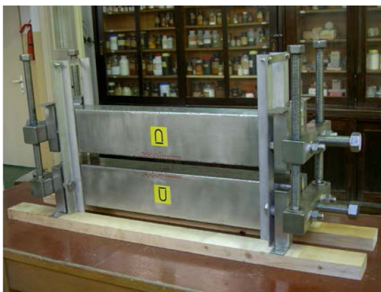
Fig. 5. (Color online) The device for the creation of the opposing assemblies from large magnetic blocks.
