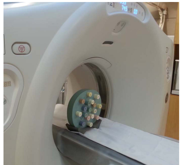
Fig. 2. (Color online) Gammex 467 tissue characterization phantom was scanned using dual CT.
