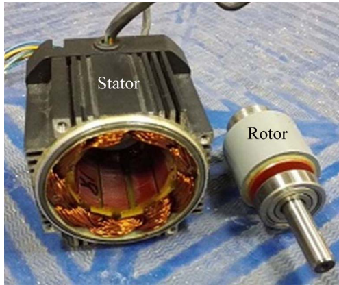
Fig. 1. (Color online) 9-slot, 10-pole fractional slot with concentrated winding BLDCM.
