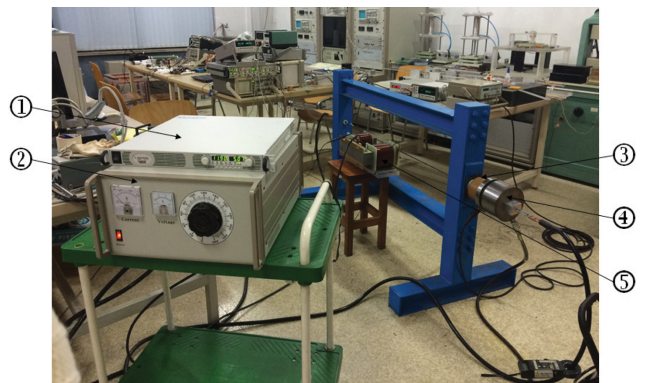
Fig. 1. (Color online) Photograph of the measuring yoke system constructed in this work; ① dc power supply, ② ac power supply, ③ load cell, ④ oil piston, ⑤ yoke apparatus.
