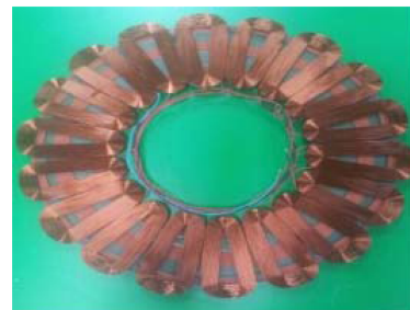
(b) Coreless windings
