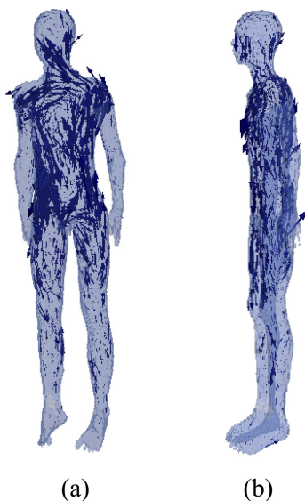
Fig. 3. (Color online) 3D distribution of induced electric field for “Louis” model at 1 MHz. (a) F2B exposure, and (b) S2S exposure.
