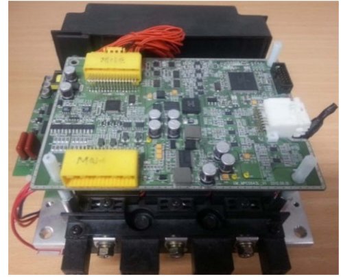
Fig. 8. (Color online) Controller of WRSM prototype (DC bus voltage: 115 V).
