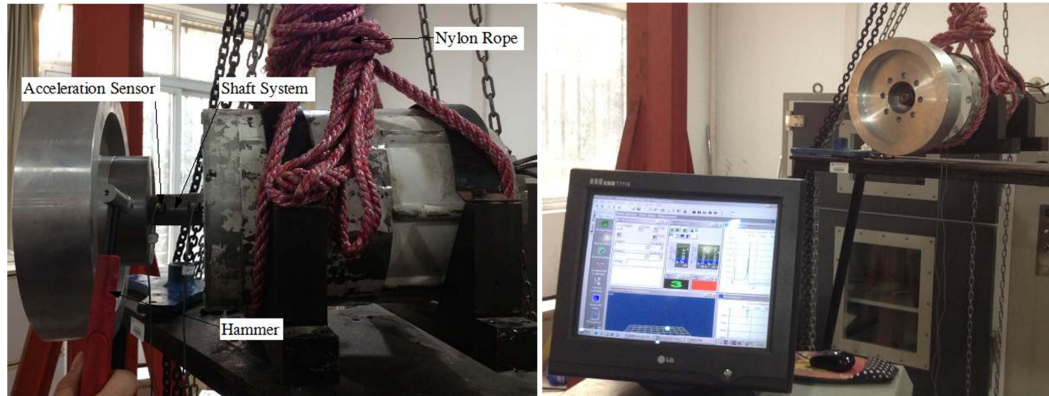
Fig. 22. (Color online) Experiment of natural frequency of the rotor system.
