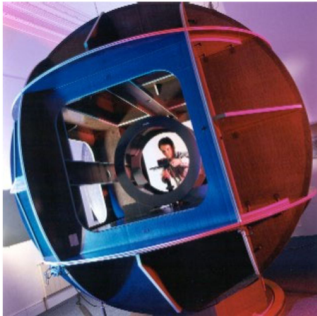
Fig. 1. (Color online) 3m diameter Helmholtz coil used to reduce the ambient magnetic field at NPL. A 1 m diameter Helmholtz coil used to calibrate magnetometers can be seen in the centre.
