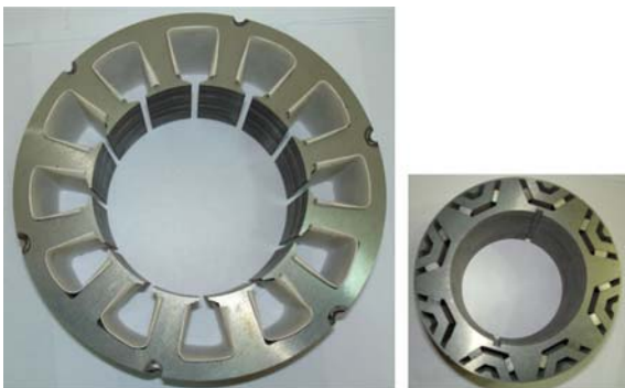
Fig. 11. (Color online) Stacked lamination stator, rotor core and inserted PMs.
