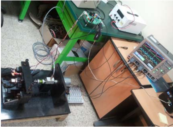
Fig. 12. (Color online) FSRM torque ripple measurement on the dynamometer.
