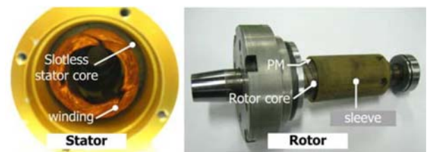
Fig. 4. (Color online) Manufactured model of slotless PM motor.
