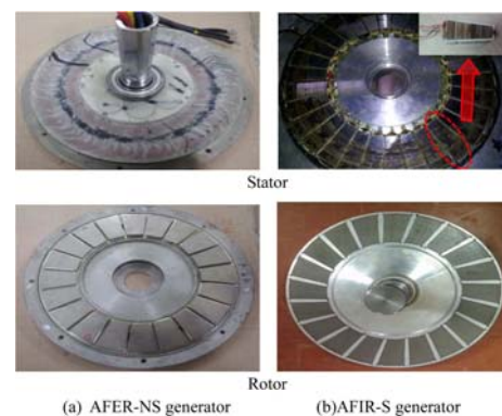
Fig. 9. (Color online) Prototypes of AFER-NS generator and AFIR-S generator having the same electromagnetic volume.
