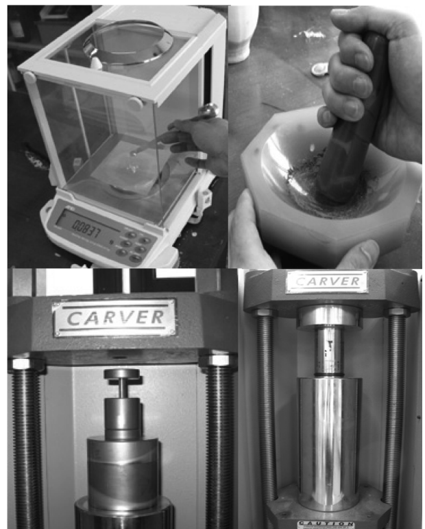
Fig. 1. Equipment and tools for the solid state reaction method (balance, mortar/ pestle, press die, press, and CIP tools).
