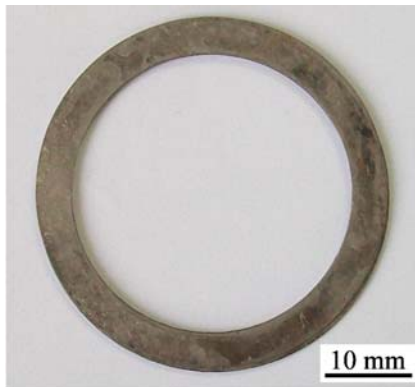
Fig. 1. Ring shape core for magnetic measurements for the cold rolled Fe-6.5%Si alloy sheets.
