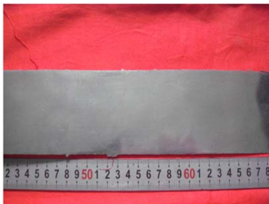
Fig. 2. The cold rolled Fe-6.5%Si alloy sheet with a thickness of 0.30 mm and width of 90 mm.
