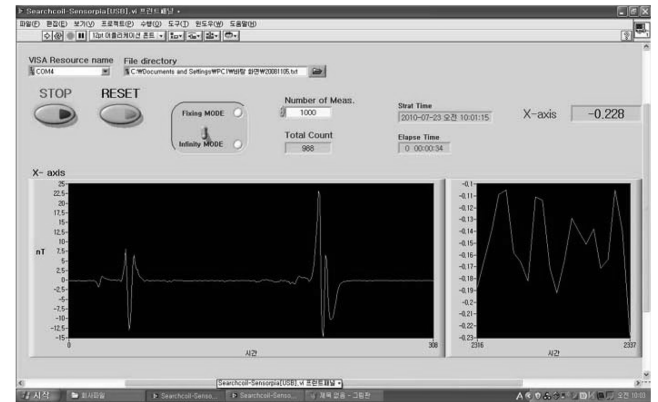
Fig. 8. LabVIEW display panel of search coil magnetometer.
