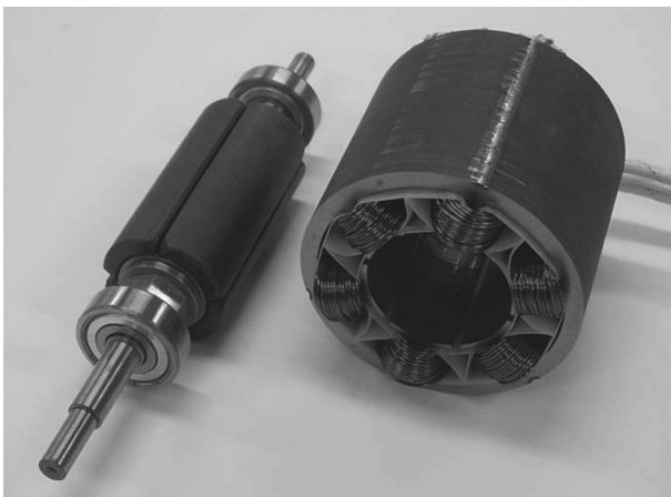
Fig. 11. Constructed prototype BLDC motor.
