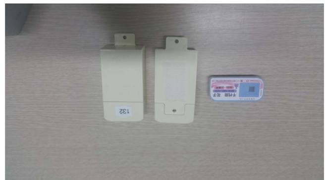
Fig. 4. (Color online) Exterior and internal structure of glass dosimeter for measuring leakage dose per week of environmental radiation.
